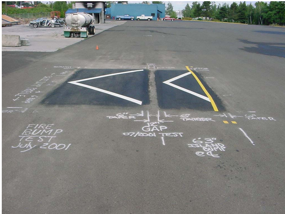
Photo 2. Offset Speed Hump with Channel Test Object – Looking Upstream.
