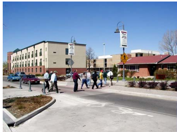
In Grand Junction, Colorado this flat-topped speed table (above) creates a level surface for pedestrian and trail crossings. Speed tables, such as this one, can be applied as the only traffic calming feature. As shown below speed tables can also be used in combination with medians, curb extensions and other treatments.
