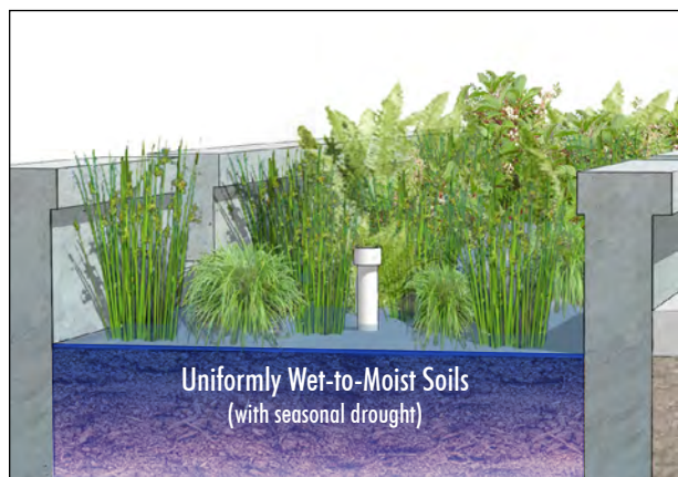
Planting conditions for LIDA facilities without sloped edges (such as concrete flow-through planters and infiltration planters) are largely uniform.
