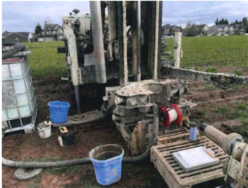
Conducting Infiltration Testing Inside 6-Inch Sonic Casing
