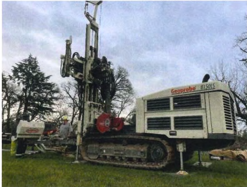
Sonic Drill Rig Soil Borings
