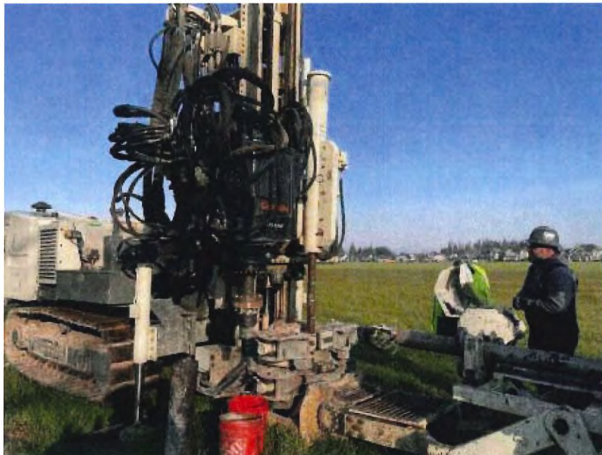
Sonic Drill Rig Soil Borings, SPT Testing
