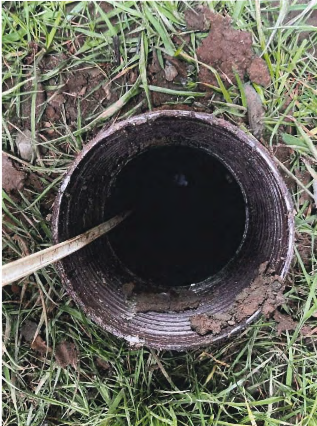
Conducting Infiltration Testing Inside 6-Inch Sonic Casing
