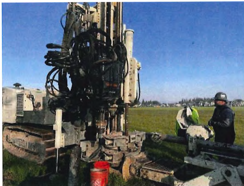
Sonic Drill Rig Soil Borings, SPT Testing
