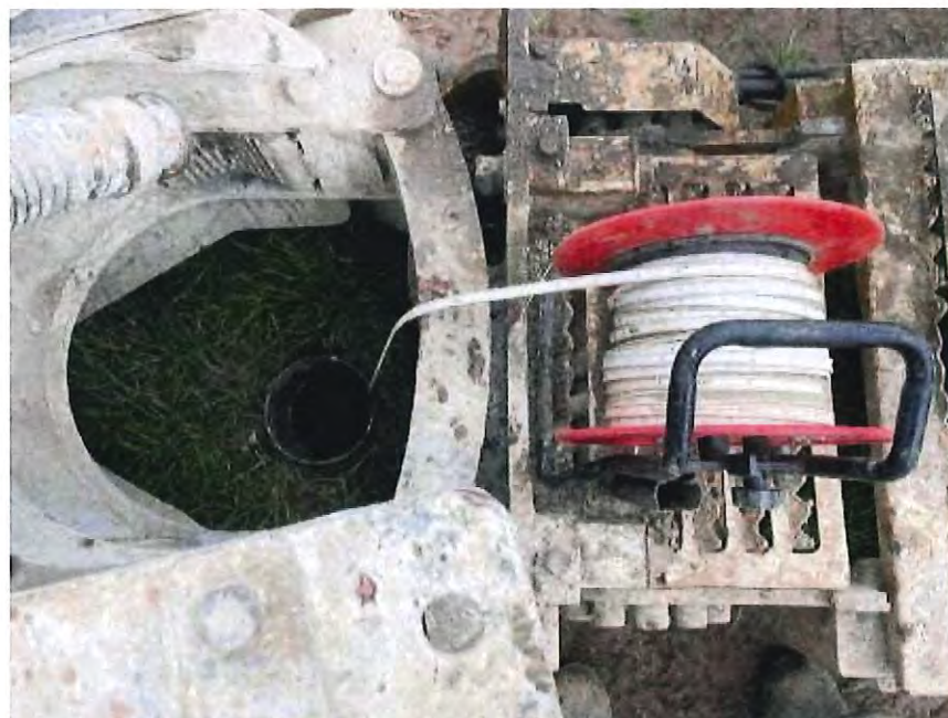
Conducting Infiltration Testing Inside 6-Inch Sonic Casing
