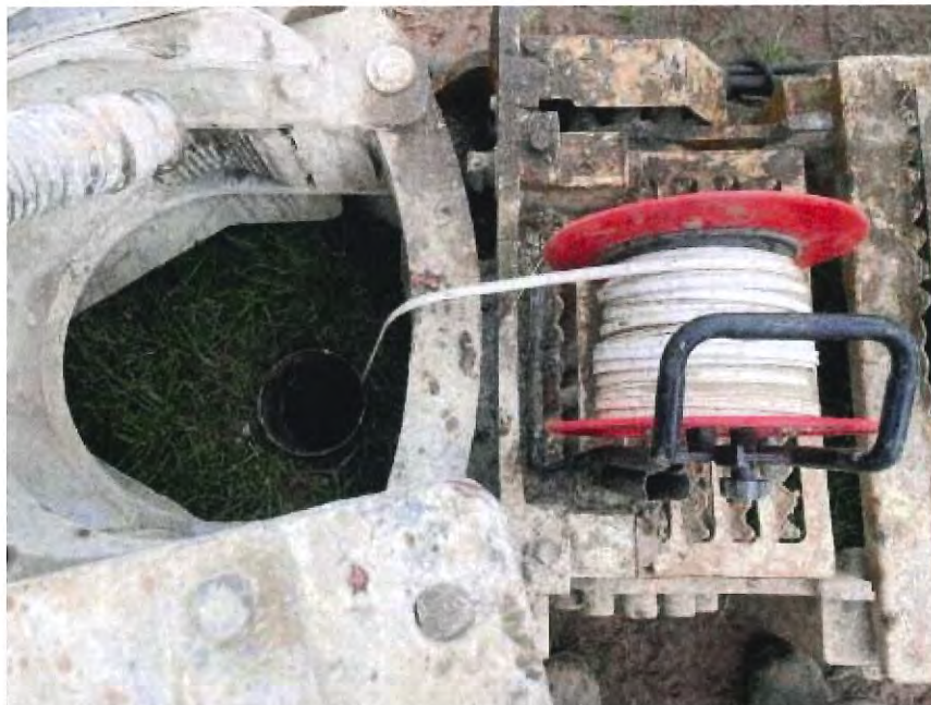
Conducting Infiltration Testing Inside 6-Inch Sonic Casing
