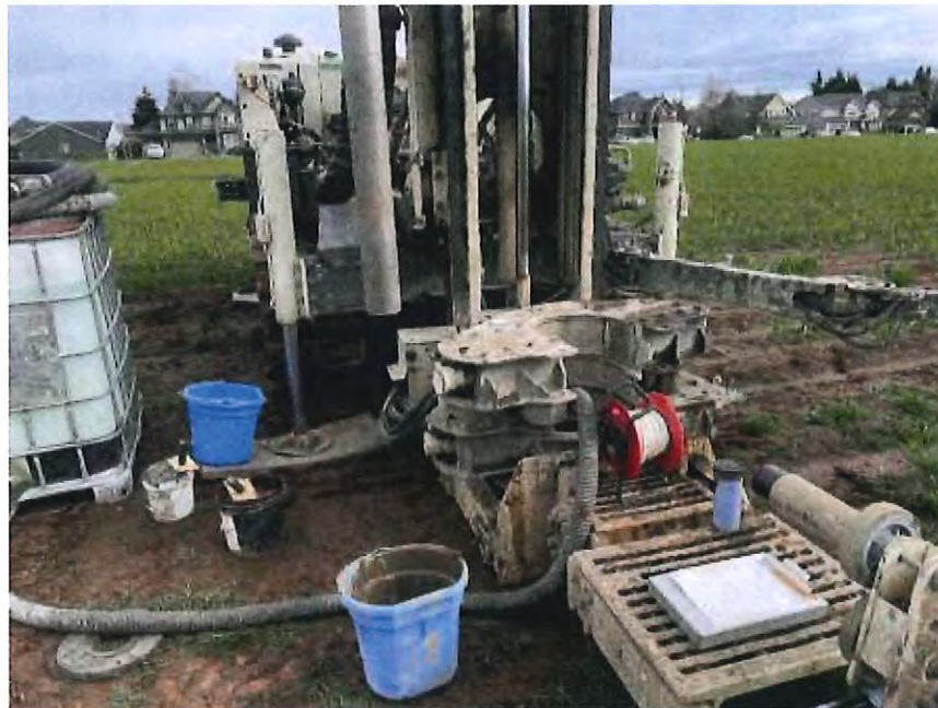
Conducting Infiltration Testing Inside 6-Inch Sonic Casing
