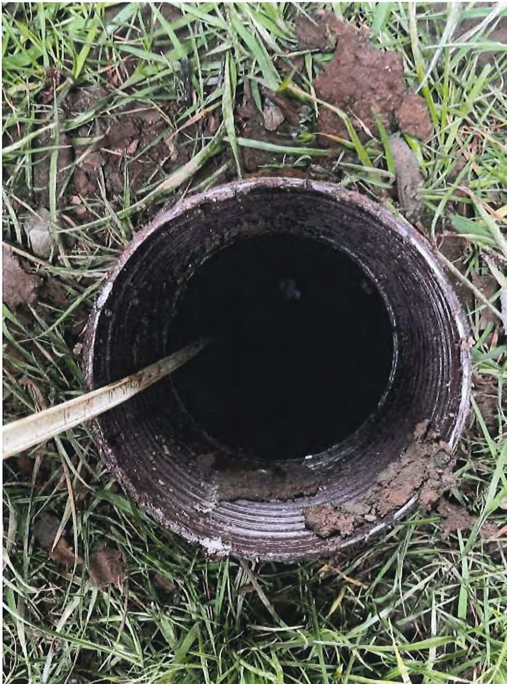
Conducting Infiltration Testing Inside 6-Inch Sonic Casing
